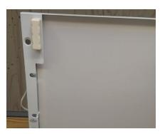
The alarm is operated with a magnet. That is why it is very important that the distance between the alarm and the magnet is not more than 10 millimetres. Place the magnet as closely to the alarm as possible. 3
