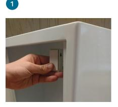
Remove the protective foil from the tape at the back of the alarm. Position the alarm in the top right corner of the cabinet with the ON/OFF switch to the right (see photo).
