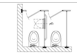
5900 Series Combination Units are to be installed so that doors open 90° to fill product maintain waste container.
