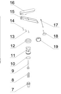
\* NOTE - Valve Body Assemblies include: Top Lever, Carry Handle, 3 x Rivets, Valve Body, Gauge, Valve Body Collar, O-Ring, Pull Pin & Retaining Strap
