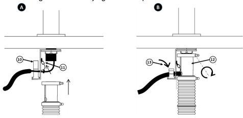
Check the installation so that the IR sensor cables or the ground are not visible, the corrugated tube must completely protect them.
