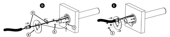
Check the installation so that the IR sensor cables or the ground are not visible, the corrugated tube must completely protect them.
