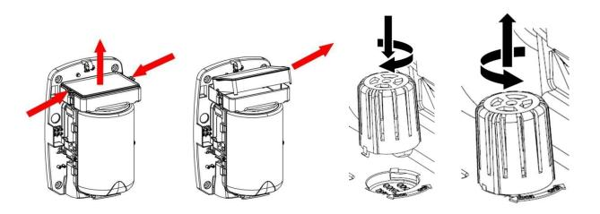
• The condition of the filter must be checked periodically.
