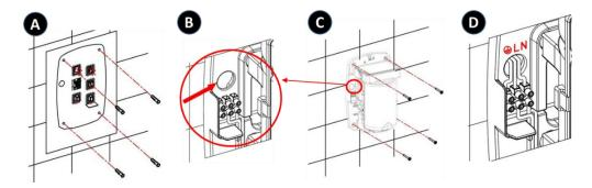
When making these connections contemplate means for disconnecting from the power grid with a minimum contact separation of at least 3 mm (0,12") for all poles. These disconnection means must be incorporated into the fixed installation. The hand dryer must be installed against a solid surface only (wall, partition, or similar).
